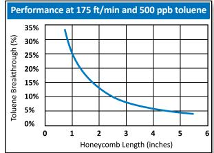
The graph above shows VOC removal using 500 ppb toluene at 175 ft/min. Toluene is a good indicator of VOCs with a vapor pressure <26 mmHg.
